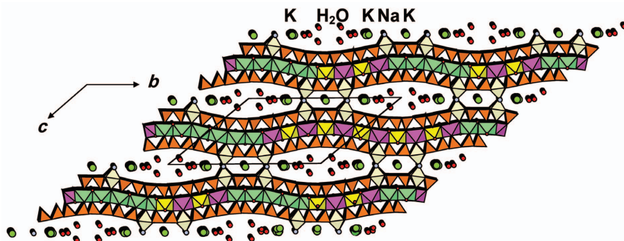
FIG. 3. General view of the crystal structure of veblenite. Si tetrahedra are orange, \text{Fe}^{2+} -, \text{Fe}^{3+} - and Mn-dominant M octahedra are green, yellow and pink, (Nb,Ti) D octahedra are pale yellow; K- and Na-dominant A(1), A(2) and B sites are shown as green and blue spheres, respectively; OH and \text{H}_2\text{O} groups are shown as small and large red spheres. The unit cell is shown with thin black lines.
